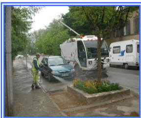
2) Millennium Plus, suction sweeper + street washer 3.5 cm hopper + 1500 l Hybrid version (mod. NA4M4 plus, NA4M6 plus))
